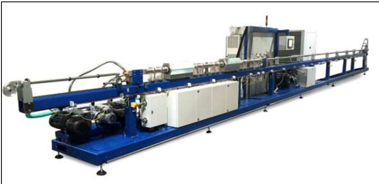
Figure 10. PlasmaANNEALER for annealing or stress relieving tubes with OD range of 6mm to 12.7mm with max output of 250kg/h.
