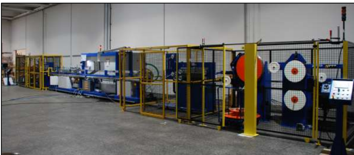
Figure 9. PlasmaANNEALER line for nickel alloy and stainless steel tubes of 0.6mm – 8.5mm OD with inlet and outlet caterpillars, double payoff and takeup (coil + spool).
