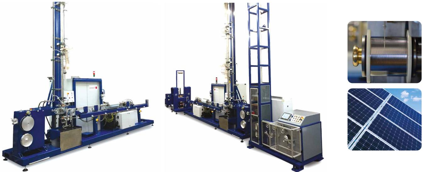
**High-speed tinning and annealing of copper or aluminium wire, tube, strip or PV ribbon**
