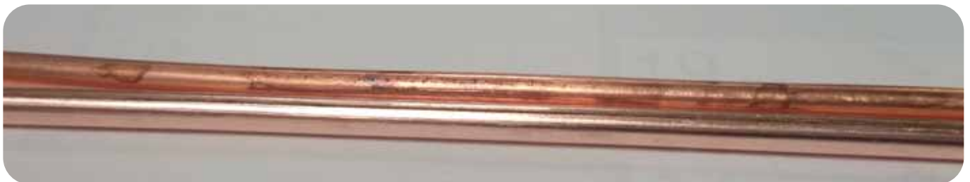
Copper wire before and after PlasmaPREPLATE treatment
