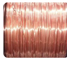
Plasma treated copper wire
