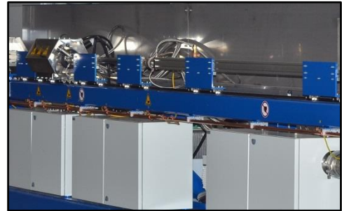
Figure 7. PlasmaANNEALER for ultra-fine SS wire dia. below 0.1mm (0.004”) for annealing in-line with drawing.
