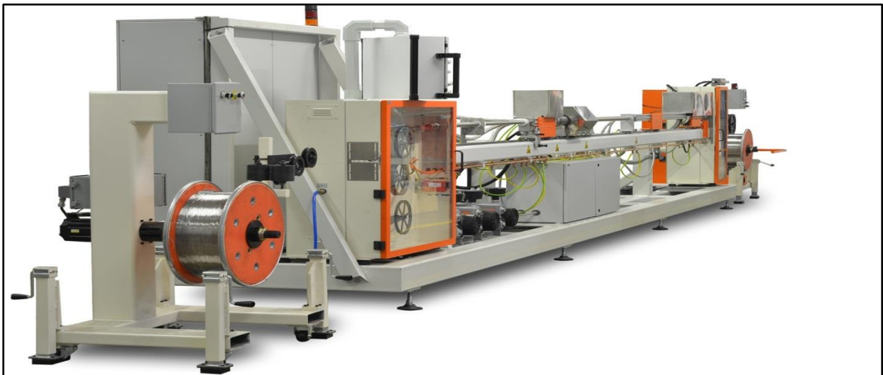
Figure 10. PlasmaANNEALER for annealing, and degreasing of stainless steel medical tubes.
