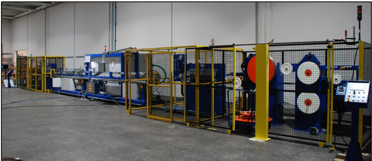
Figure 11. PlasmaANNEALER line for nickel alloy and stainless steel wire and tubes of 0.6mm - 8.5mm OD with inlet and outlet caterpillars, double takeup (coiler + spooler).
