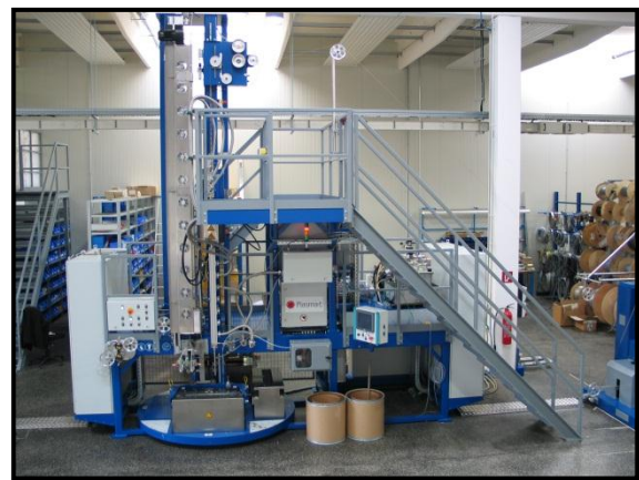
Figure 3: Plasma annealer as part of copper wire or tube tinning line
