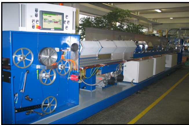
Figure 2: Plasma annealer for stainless steel tube with inbuilt transport system
